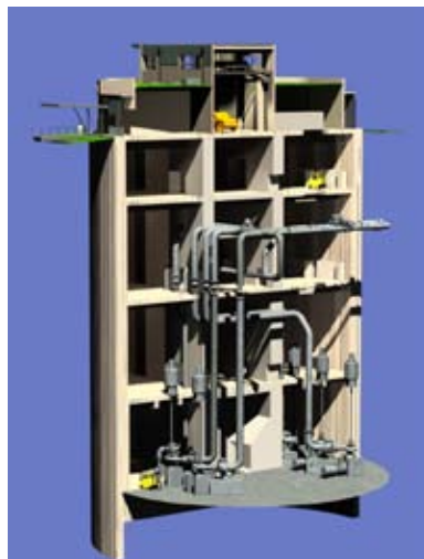
Portland's 220-mgd Swan Island Pump Station will pump combined sewage to the Columbia Boulevard Wastewater Treatment Plant.
