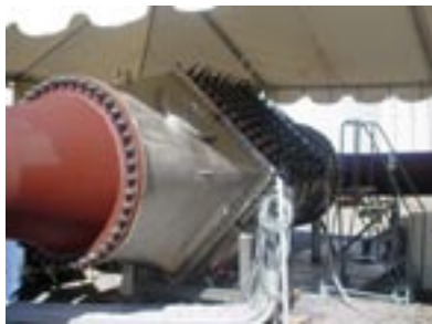
Validation of a 40-mgd UV reactor moves large-scale UV from research to practice.
