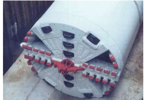
Varying soil conditions required the use of three different MTBM cutter heads.
