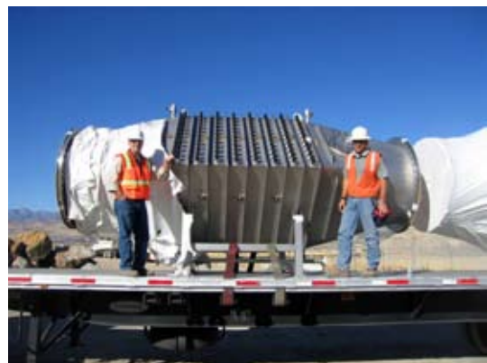
Carollo provided construction services for the installation of large-scale WEDECO K143 reactors validated to flows of 40 mgd.
