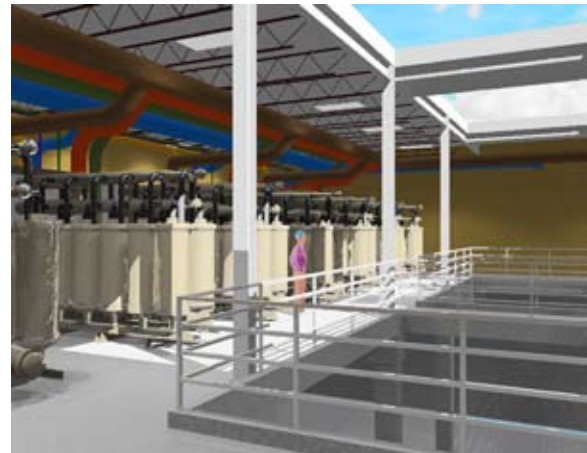
The City of Lake Forest retained Carollo to design new ultrafiltration membranes at its water treatment facility to protect consumers from water-borne pathogens.
